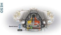
An industry first, our exclusive Honda Electronic Steering Damper (HESD) senses bike speed and acceleration and adjusts damping force accordingly. At low speeds an electronically controlled relief valve is open for lighter steering. Speed up, and the valve adjusts for increased damping force.
